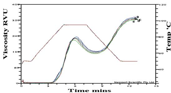
**Figure 3.** Pasting properties of rice flours with different particle sizes. Samples are indicated as: a ( $\leq 63 \mu\text{m}$ ); b ( $80 \mu\text{m}$ ); c ( $100 \mu\text{m}$ ); d ( $125 \mu\text{m}$ ); and e ( $140 \mu\text{m}$ ).
