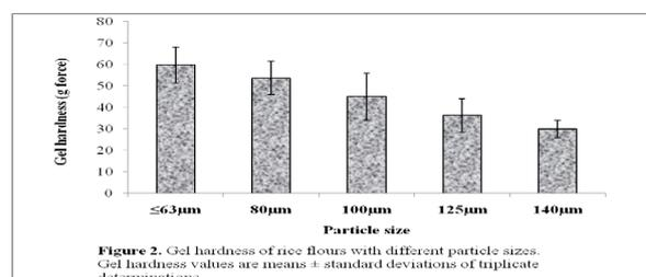
**Figure 2.** Gel hardness of rice flours with different particle sizes. Gel hardness values are means  $\pm$  standard deviations of triplicate determinations.
